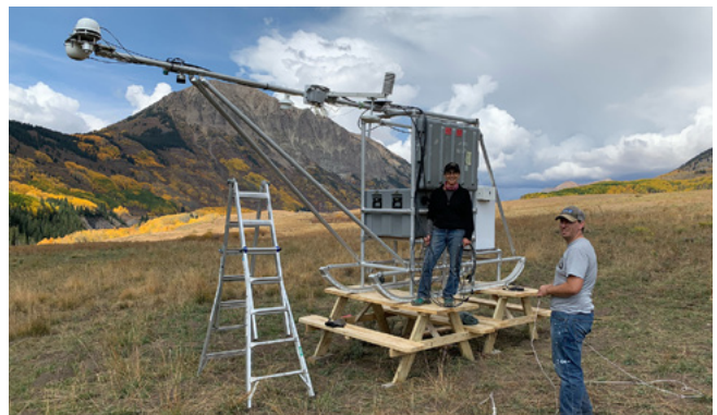
Janet Intrieri and Chris Cox, from NOAA Research's Physical Science Laboratory, install an Atmospheric Surface Flux Station for SPLASH. Photo credit: Gijs de Boer, NOAA/ Cooperative Institute for Research in Environmental Sciences
